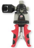
The Series HCHP Hydraulic Calibration Hand Pump utilizes a fully adjustable stroke control that allows for quick priming, easy pumping, and fast pressure generation up to 10,000 psi (700 bar). The ergonomically engineered handles provide extra comfort, while the triple filtration system ensures pump operation in spite of dirty conditions.
